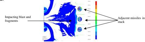
Figure 5 – Adjacent stack reaction
