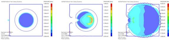
Figure 3 - Fragment impact on a missile in its container
